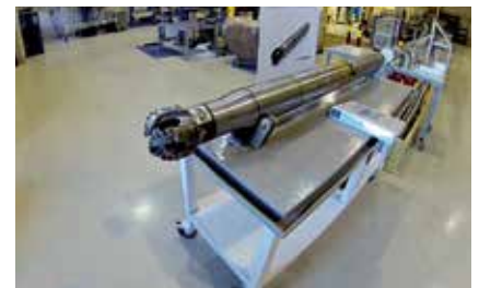
Badger Explorer has been test run in a DEMO 2000-supported demonstration project. Here is the 30-metre-long drilling robot at the workshop in Stavanger. Photo: Badger Explorer
