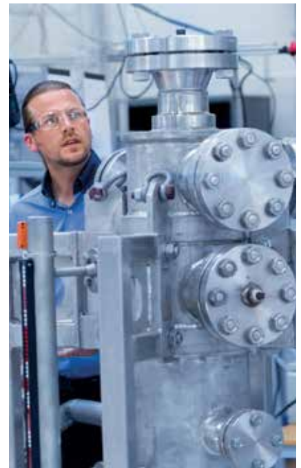
The new separators are much more compact than the traditional gravity based separators. Photo: Sverre Jarild
