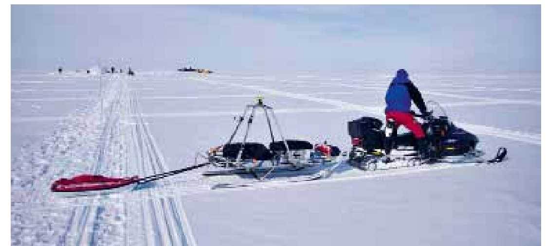
Snow radar and GPS elevation profiling at the summit of Austfonna Ice Cap. Photo: Jon Ove Hagen
