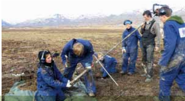
UNIS students and Professor Bo Elberling hand drilling into permafrost in Zackenberg, NE Greenland. Here they are starting to obtain the core sample. Photo: Hanne H. Christiansen
