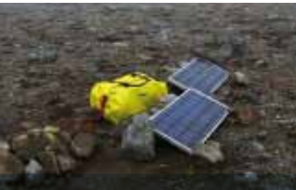
Instruments and solar panels for one of the 13 elements of the seismic array on Bjørnøya. Photo: Johannes Schweitzer
