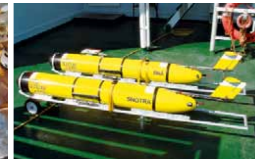
Autonomous “gliders” on deck. Photo: Ken Drinkwater
