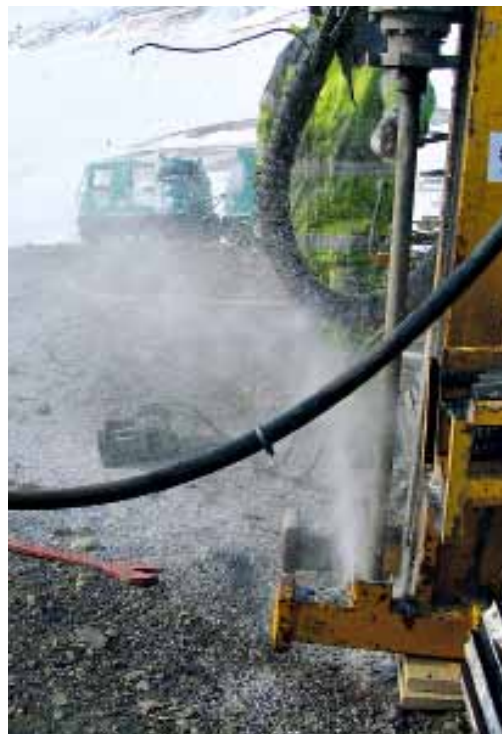
The hammer drill rig bores into an ice-rich pingo on Svalbard. Photo: Hanne H. Christiansen
