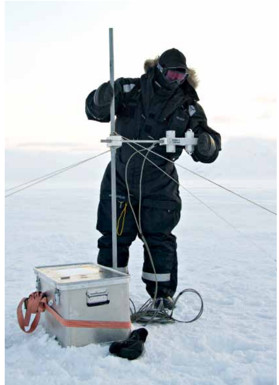
Measuring albedo – how much a surface reflects solar radiation – in Adventdalen valley. Photo: Erik W. Kolstad
